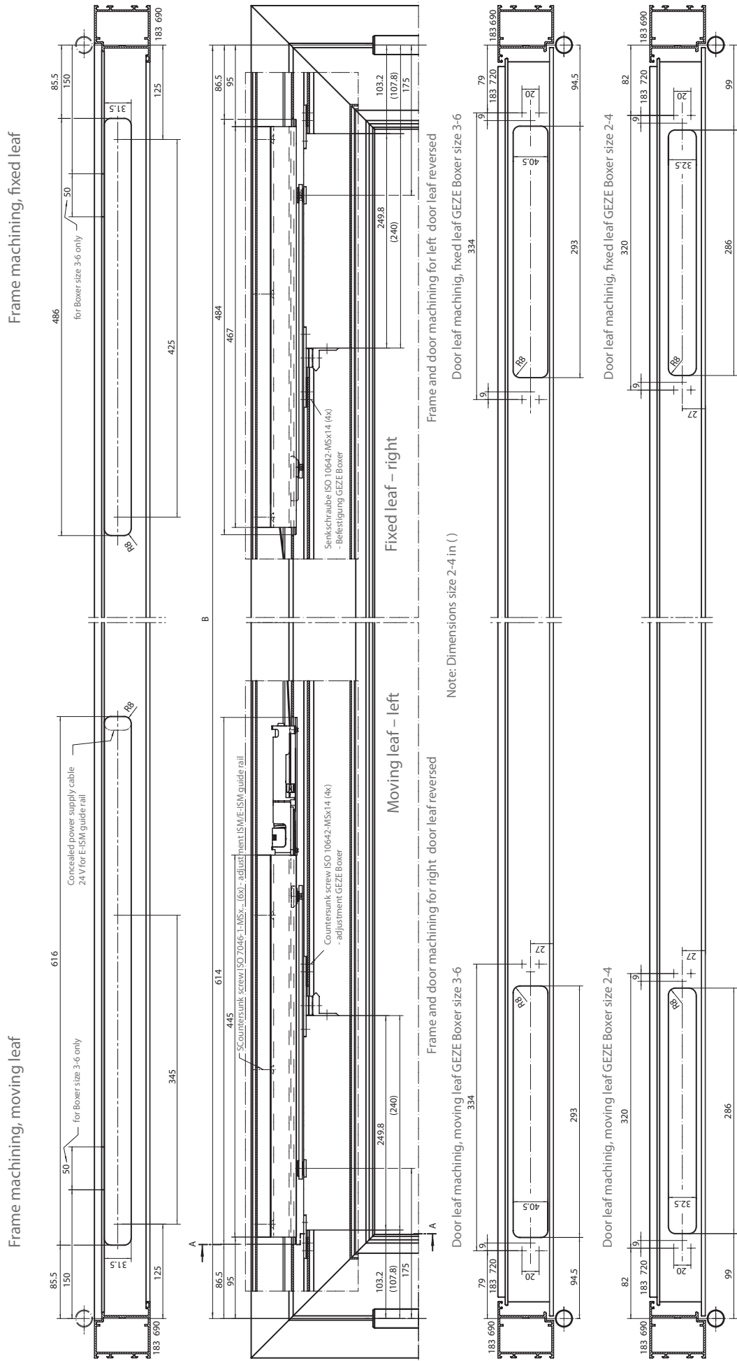
Fig. 14-1 · ISM/E-ISM guide rail Boxer size 2-4/3-6, aluminium door
