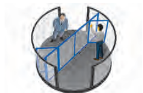
Two-wing automatic revolving doors ← The door wings of two-wing doors are fixed to the H-girder which can drive the door wings.
