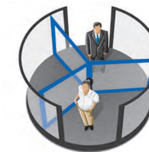
Three/Four-wing revolving doors ← The door wings of the three/four wings revolving doors are fixed to the central axis which can drive the door wings.
