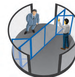
Two-wing automatic revolving doors ← The door wings of two-wing doors are fixed to the H-girder which can drive the door wings.
